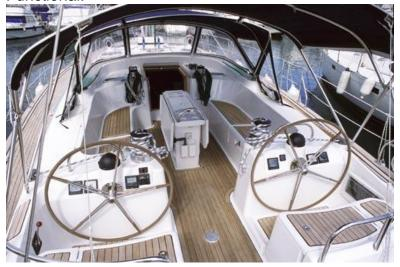
2170 Upper deck Functional. White gel coat with molded in non-skid. Condition is serviceable.
